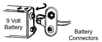
Figure 1 : Attaching battery to the battery snap
